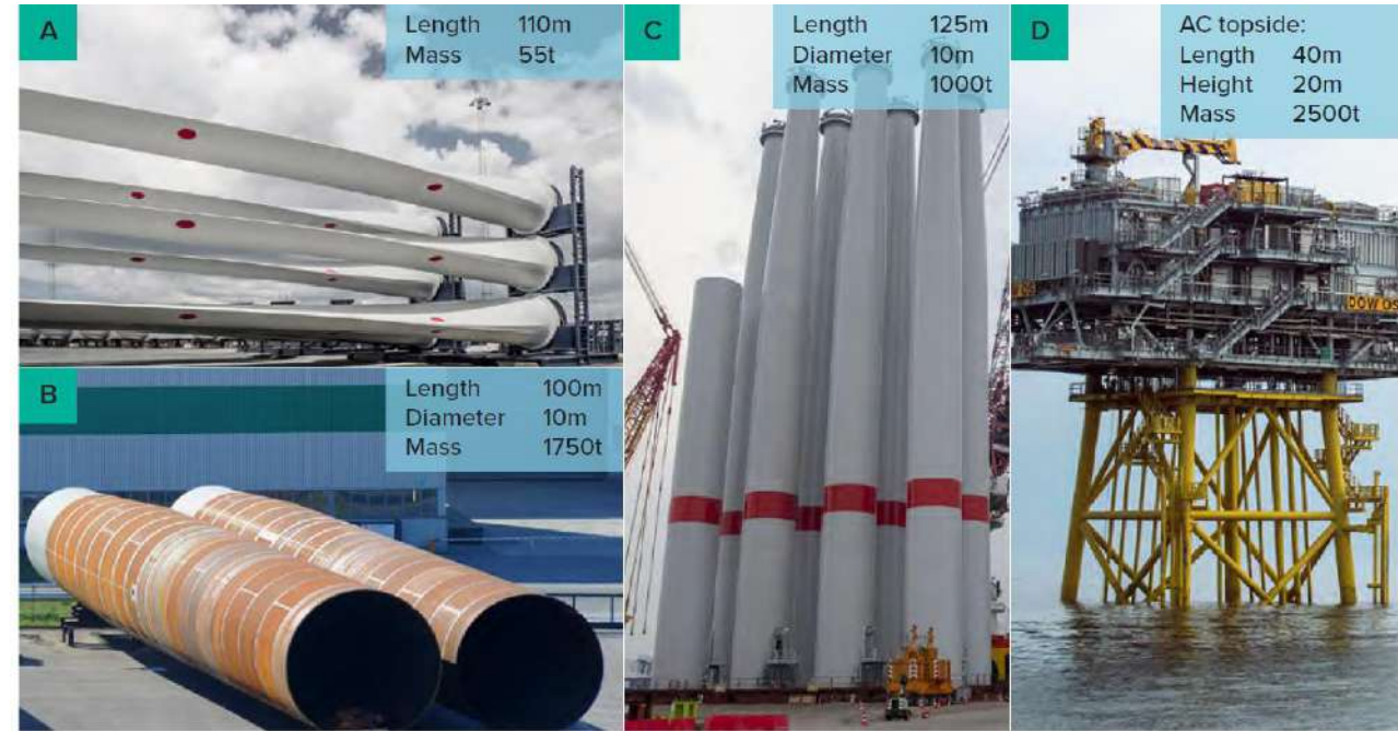
Representative dimensions for next-generation 15 MW-scale turbines
